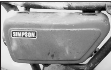
XS/TX650 1974-79 "Standard" Type 1 3/8" Wide bracket for side cover damper rubber (upper) Hanger Side covers are steel.
