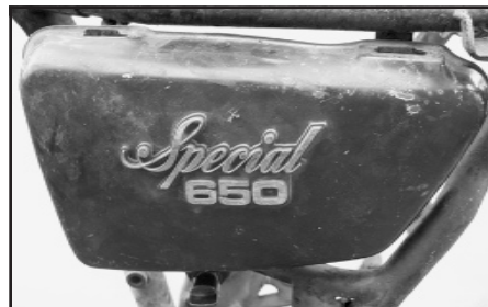
XS650Se/Sf/2F/G 1978-80 "Special" Type 1" Wide bracket for side cover damper rubber (upper) Hanger Side covers are steel.
