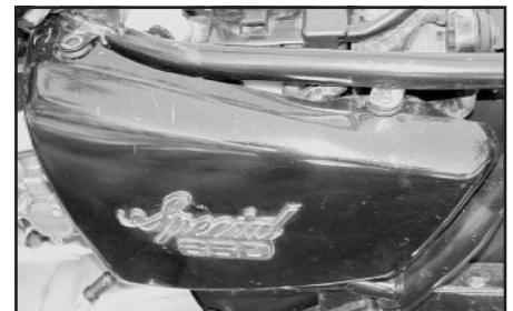
All 1980-84 (except 80G) Type Grommet mount damper rubbers used on upper & lower mount points. Side covers are Plastic.
